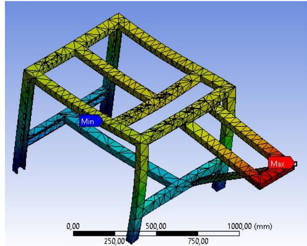
Figure 5: Deformation total of chassis
