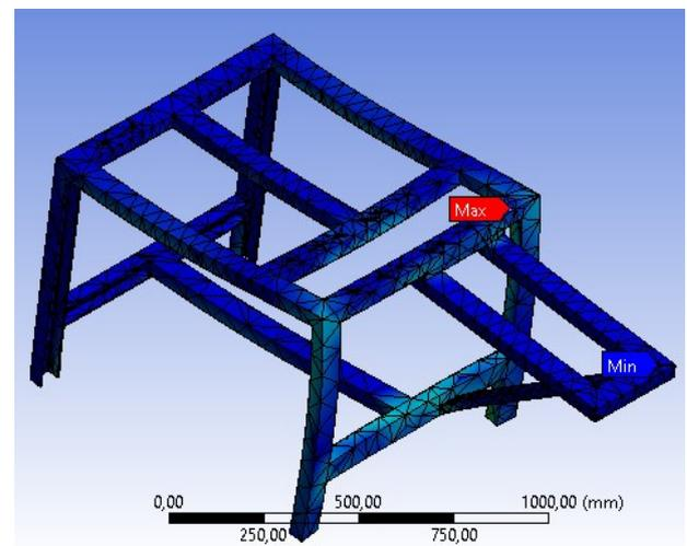
Figure 6: Total of chassis equivalent strain
