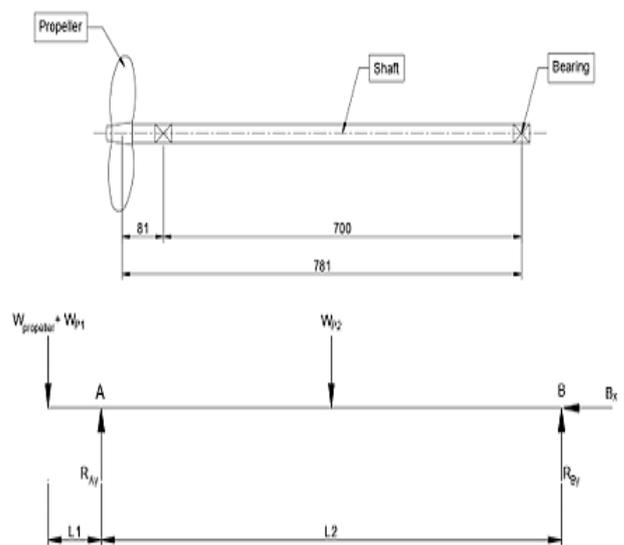
Figure 3: Free body diagram of shaft and propeller
