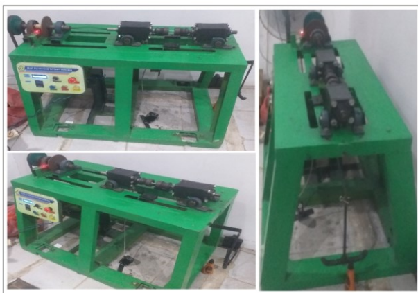
Figure 5: The rotary fatigue test equipment
