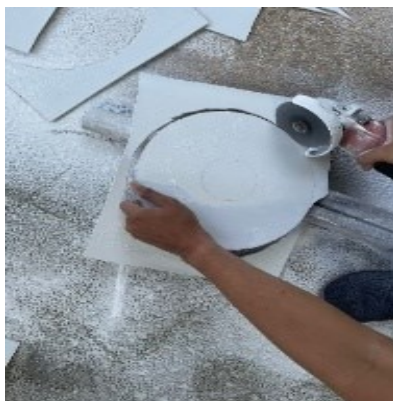
Figure 6: Pipe is shaped and cut like a circle
