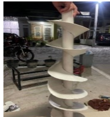
Figure 8: Blade and shaft union
