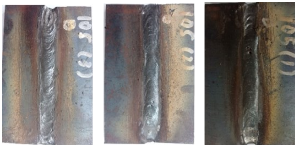
Figure 8: Welding results using the E7018 electrode at 105 A
