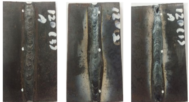
Figure 6: Welding results using the E6013 electrode at 120 A
