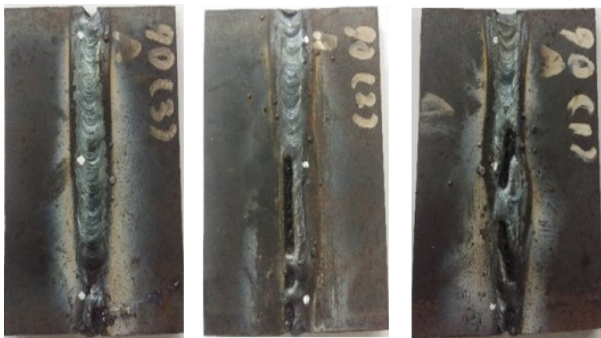
Figure 4: Welding results using the E6013 electrode at 90 A
