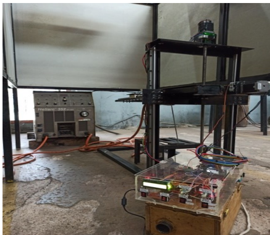
Figure 2: Two axis adaptive sliding machine with speed control
