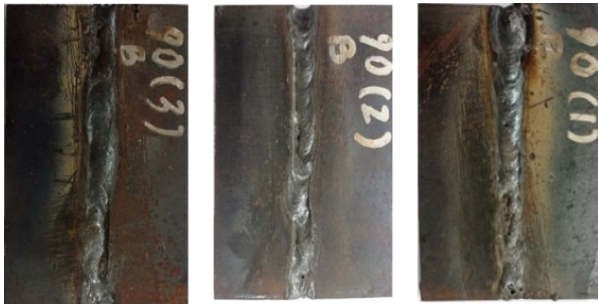
Figure 7: Welding results using the E7018 electrode at 90 A
