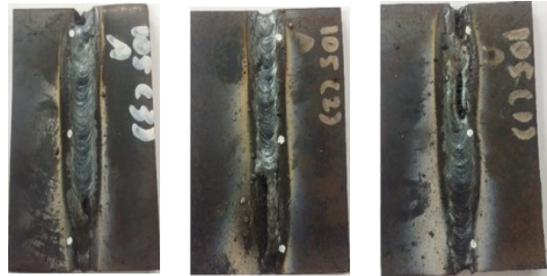
Figure 5: Welding results using the E6013 electrode at 105 A
