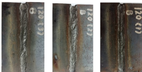
Figure 9: Welding results using the E7018 electrode at 120 A
