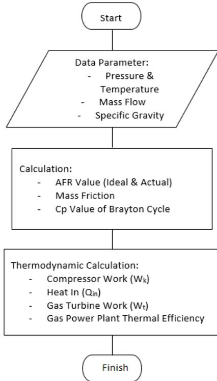
Figure 1: Energy calculation flowchart
