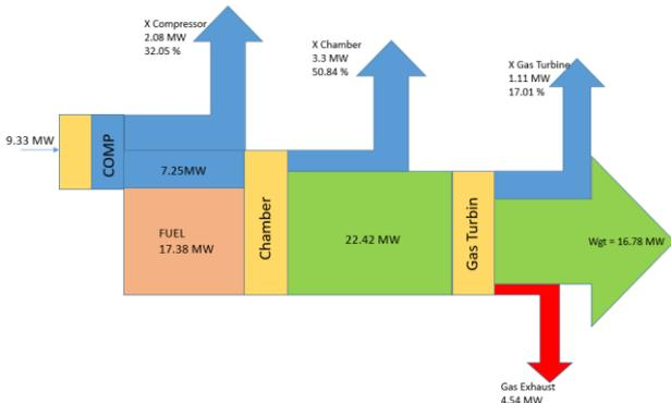
Figure 5. Grassman diagram of a gas power plant
