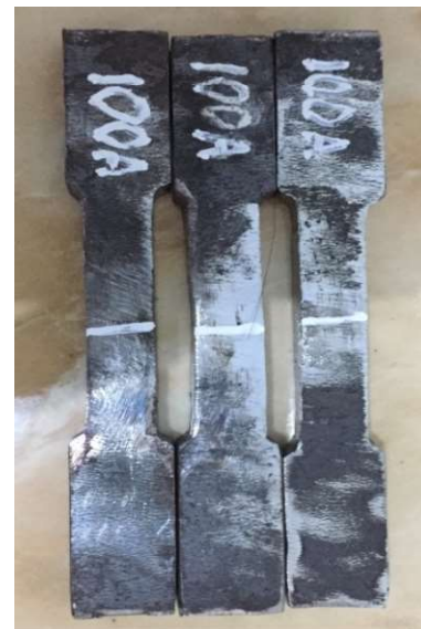
Figure 3: Specimens for tensile tests that have been welded
