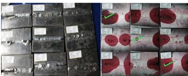
(a) The specimen welds (b) Results of liquid Penetrant Testing
