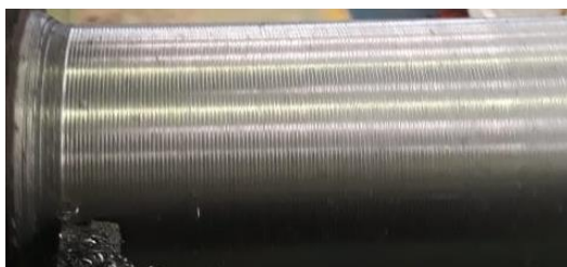
Figure 6: he roughness contour result from experiment 1
