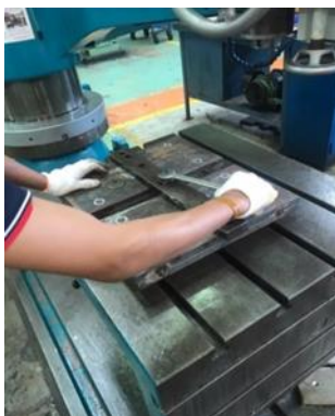
Figure 8: Clamp on the Workpiece
