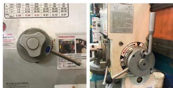
Figure 11: Adjust the Motion and Feeding Speed on the Spindle
