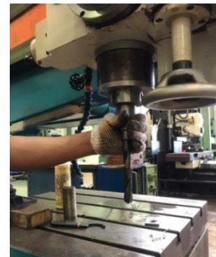
Figure 10: Installation of Drill Bit on the Spindle
