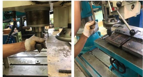
Figure 9: Centering the spindle with the workpiece
