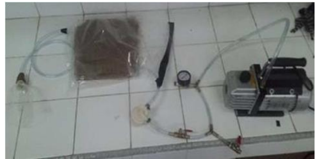
Figure 1: Vacuum assisted resin infusion (VARI)
