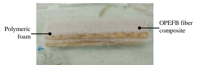
Figure 2: OPEFB fiber reinforced polymer composites-polymeric foam sandwich panels
