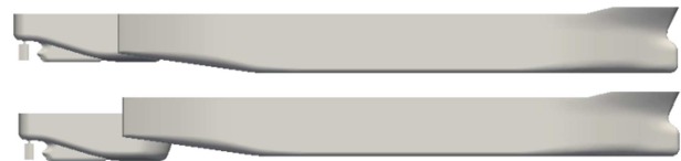
Figure 2: Overview of the pusher and the full-load barge (above) and the ballast barge (below)
