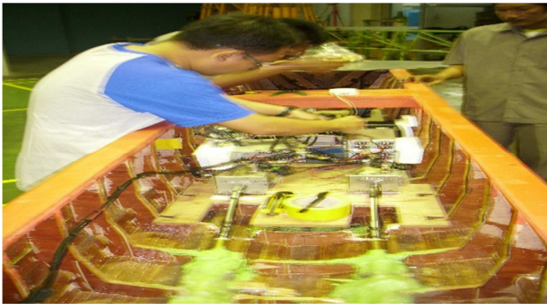
Figure 5: Installation of instrumentation equipment for seakeeping test
