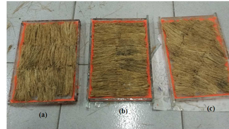
Figure 2: Direction of the OPEFB fiber arrangement
