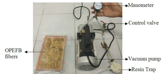
Figure 4: Vacuum assisted resin infusion
