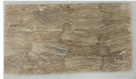
Figure 7: Polymeric composite-OPEFB fiber sandwich composite panels
