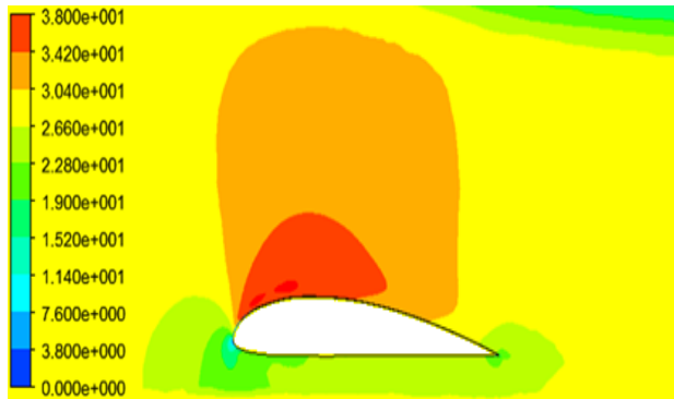
V=30 \frac{m}{s} Ribletted aerofoil
