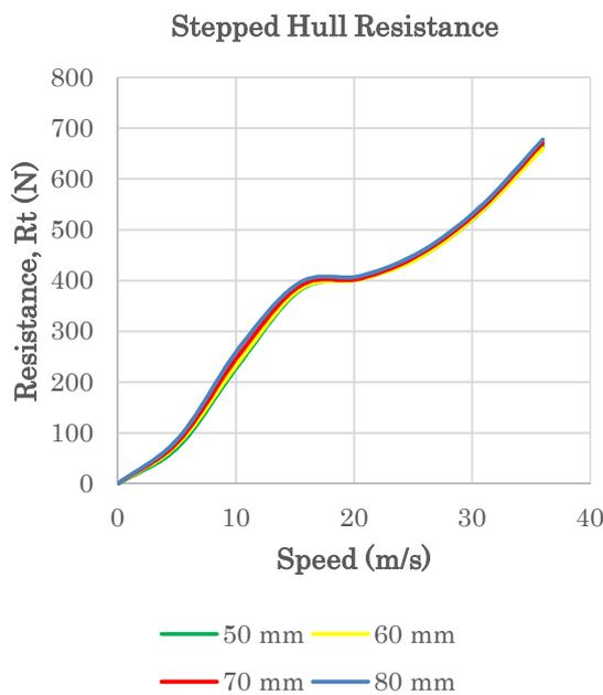
**Figure 5:** Stepped Hull Resistance at various speeds ranging from 0 to  $35.9 \text{ ms}^{-1}$
