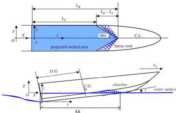
Figure 1: Length of wetted keel and chine ( $L_K$  &  $L_C$ ) (Hassan Ghassemi, et.al, 2008)
