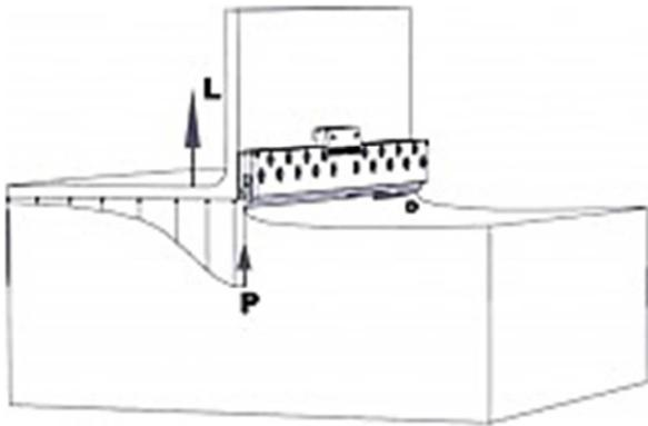
Figure 2: An interceptor plate protruding the water surface
