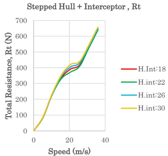
**Figure 6:** The total resistance for the stepped hull fitted with interceptor plate of heights (18-30) mm
