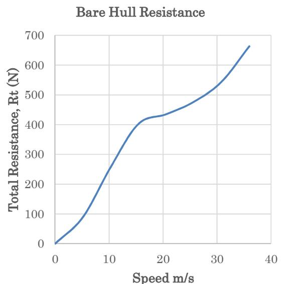
Figure 4: Resistance of the bare hull at various speeds ranging from 0 to  $35.9 \text{ ms}^{-1}$
