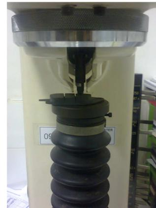
Figure 3: Hardness testing setup
