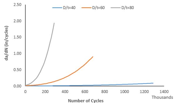
Figure 7: Growth of crack depth for three model of pressure vessel with same crack size
