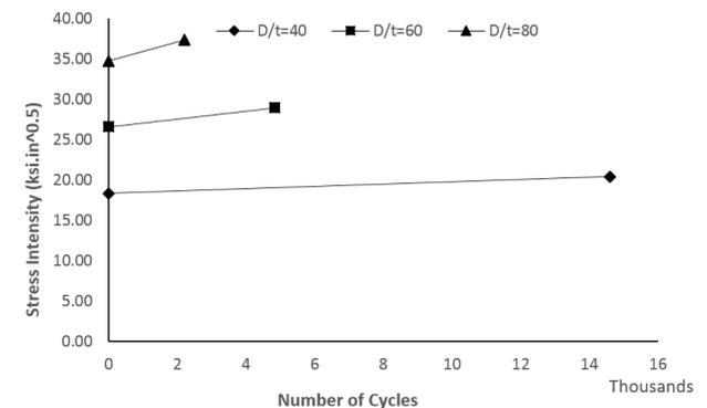
Figure 11: Stress intensity factor during crack growth for initial crack with *a/t*=0.8 and *a/c*=0.1
