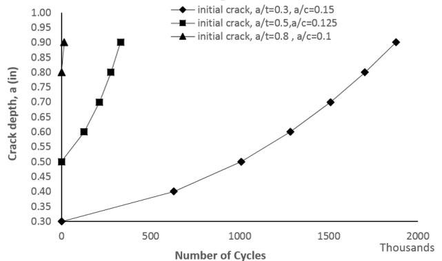
Figure 16: Increasing value of crack depth for various size of crack in pressure vessel with  $D/t=40$
