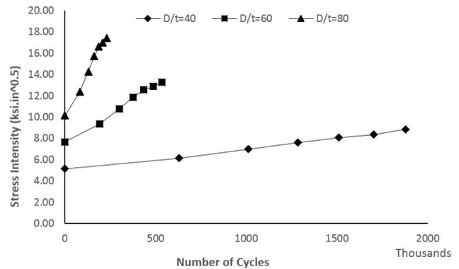
Figure 9: Stress intensity factor during crack growth for initial crack with *a/t*=0.3 and *a/c*=0.15
