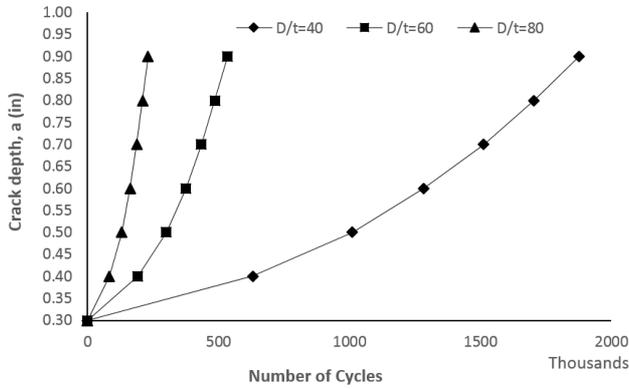
Figure 12: Depth of crack with initial value,  $a/t=0.3$  and  $a/c=0.15$ , during crack growth
