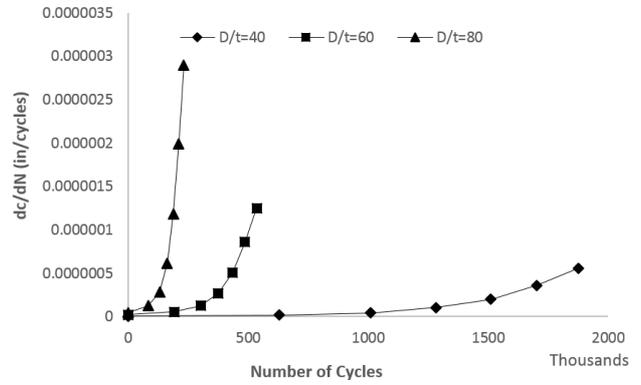
Figure 15:  $dc/dN$  of crack with initial value,  $a/t=0.3$  and  $a/c=0.15$ , during crack growth
