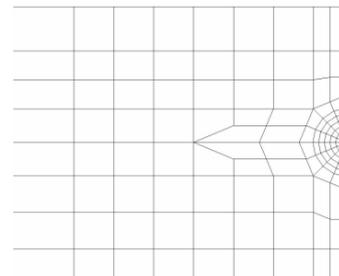
Figure 4: Spider web mesh design with elements concentrated at the crack tip [6]
