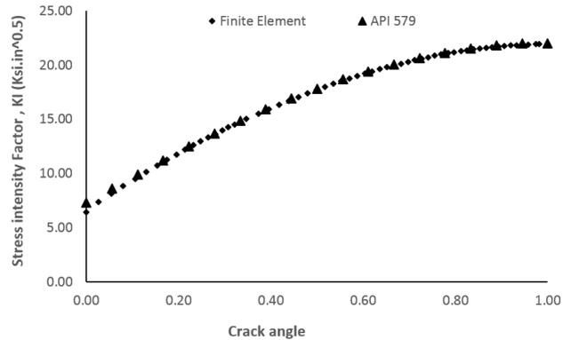
Figure 6: Validation curve for numerical model of cracked pressure vessel with D/t=60, a/t=0.4 and a/c=0.125
