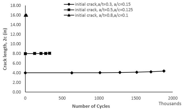
Figure 17: Increasing value of crack length for various size of crack in pressure vessel with  $D/t=40$
