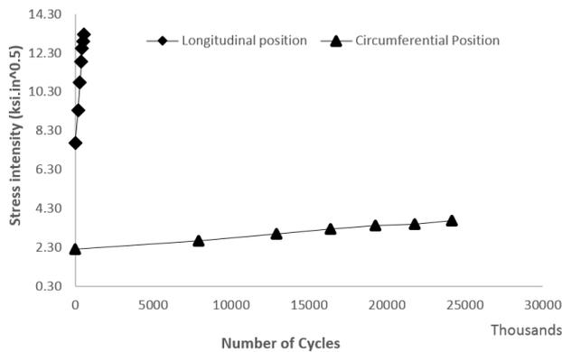
Figure 18: Stress intensity of growing crack with initial size  $a/t=0.3$  and  $a/c=0.15$  in pressure vessel with  $D/t=60$
