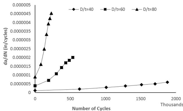
Figure 14:  $da/dN$  of crack with initial value,  $a/t=0.3$  and  $a/c=0.15$ , during crack growth
