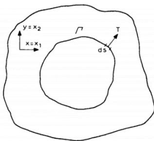
Figure 5: Definition of *J*-Integral Method [8]
