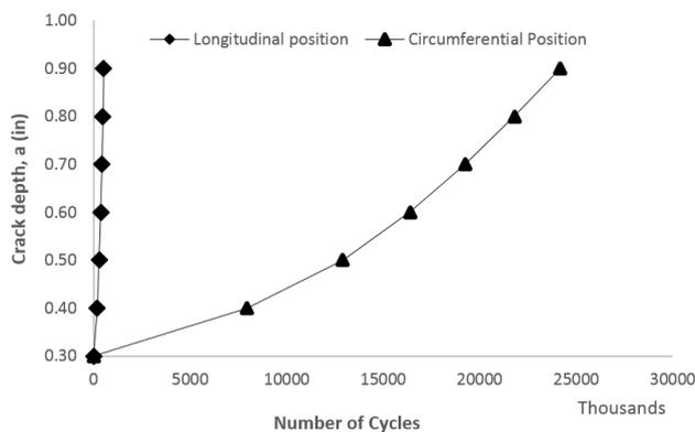
Figure 19: Crack depth of growing crack with initial size  $a/t=0.3$  and  $a/c=0.15$  in pressure vessel with  $D/t=60$
