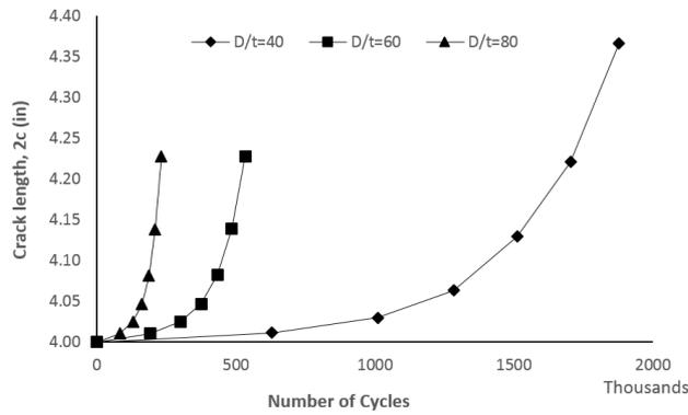
Figure 13: Length of crack with initial value,  $a/t=0.3$  and  $a/c=0.15$ , during crack growth
