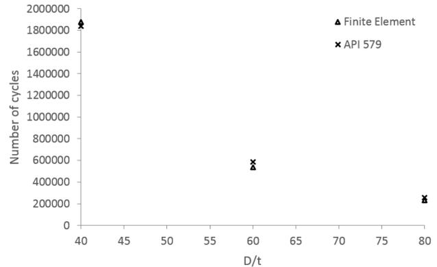
Figure 20: Comparisons of failure prediction API 579 and finite element
