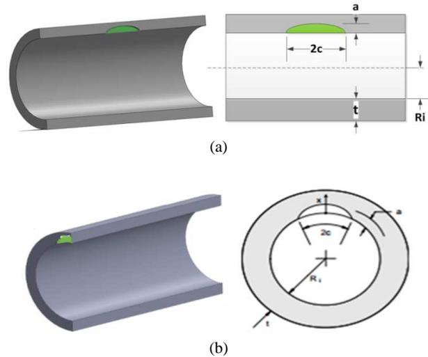
Figure 3: Position of crack in pressure vessel: (a) internal longitudinal crack, (b) internal circumferential crack
