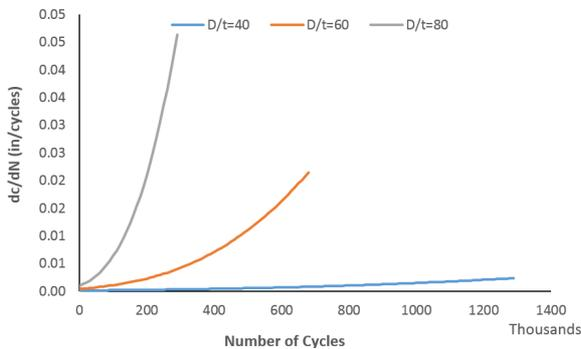
Figure 8: Growth of crack length for three model of pressure vessel with same crack size
