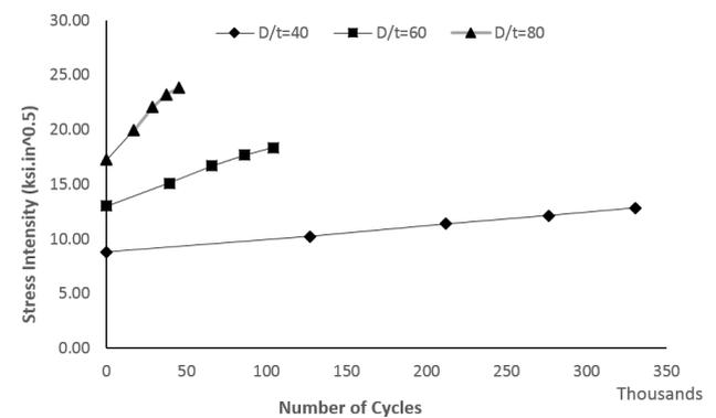
Figure 10: Stress intensity factor during crack growth for initial crack with *a/t*=0.5 and *a/c*=0.125
