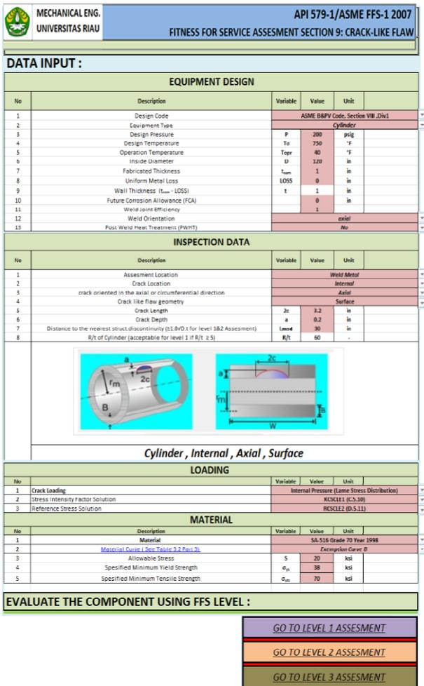
Figure 2: Screen shoot of crack growth calculation sheet program
