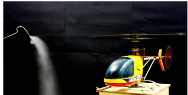
(a) Smoke released on the superficial portion of the main rotor blade during hover.
