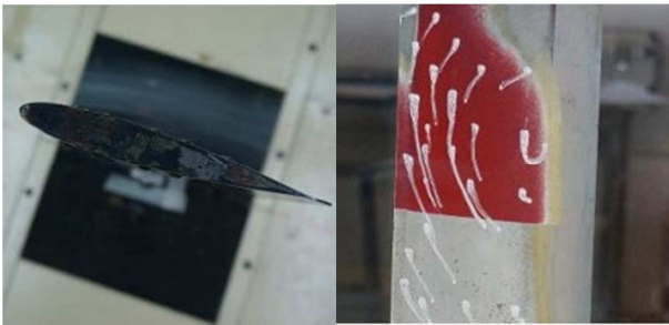
Figure 14 Smoke test and oil dot test
