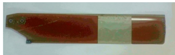
Figure 2 The generic model of tail rotor blade for Bell B206 [6]
