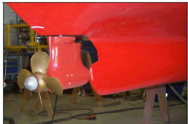
Figure 6: Stern design for model scale of Sumitomo DAT (Juurma et al. , 2012).
