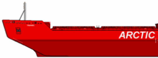
Figure 3: Ice Breaking Bow of double acting ship (Stephen, 2004)
