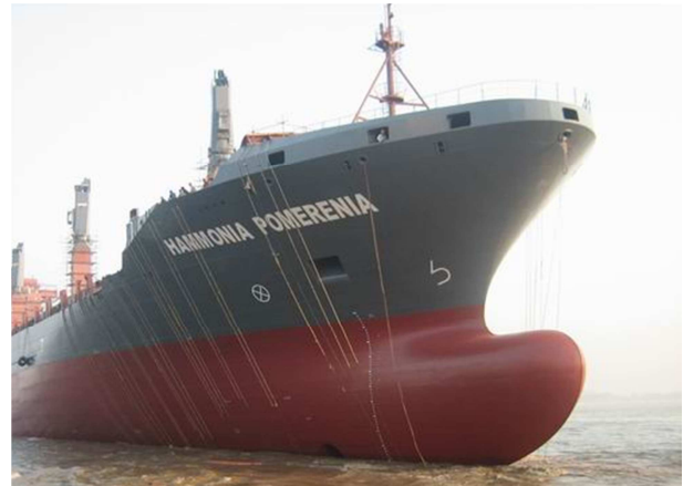
Figure 2: Bulbous bow for common tanker
