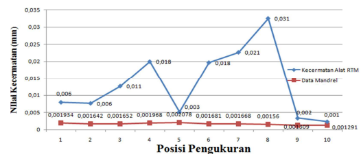
Figure 10: Graph of Accuracy Measuring roundness (Roundness Tester Machine)
