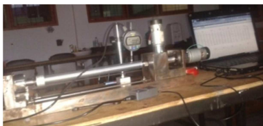
Figure 3: Measuring roundness (Roundness Tester Machine)
