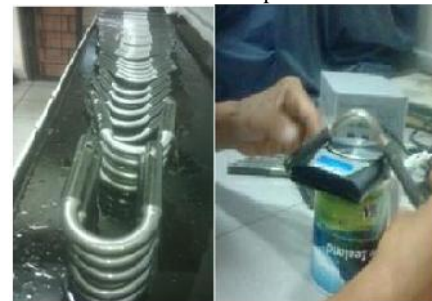
(a) (b) Figure 3.3 (a) specimens after bending, (b) Weighing before soaked
