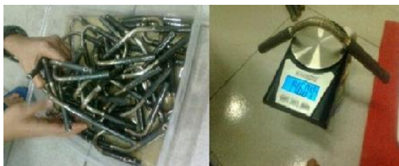
(a) (b) Figure 3.6 (a) Cleaning process, (b) Weighing after soaked
