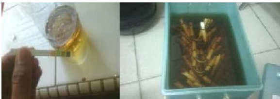
(a) (b) Figure 3.5 (a) Measuring the potential of hydrogen (pH scale) which contained, (b) The all specimen were soaked in the peat water
