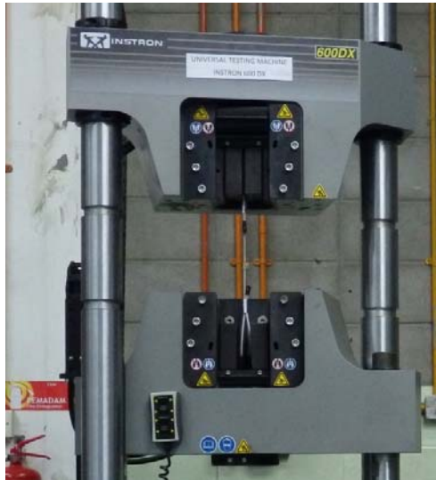
Figure 5: Wire rope tensile experiment setup
