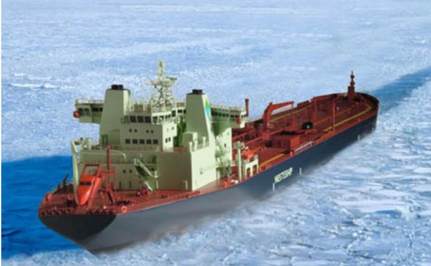
Figure 2: Double Acting Tanker Tempera in ice condition <sup>(1)</sup>
