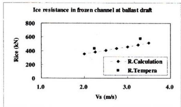
Figure 17: Ice resistance in frozen channel at ballast draft astern with propeller and then compare with existing DAT "Tempera" <sup>(4)</sup>
