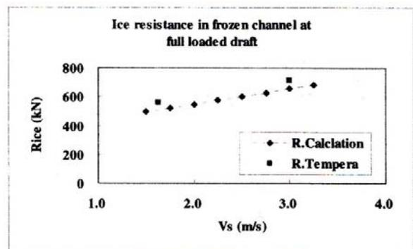
Figure 16: Comparison ice resistance of selected hull form in frozen channel at full loaded draft in astern with existing DAT "Tempera" <sup>(4)</sup>
