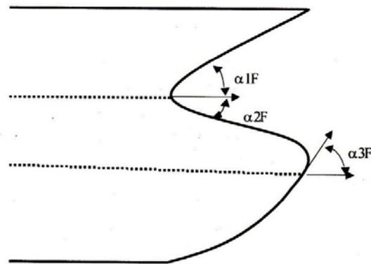
Figure 4: Two part of fore hull form modification.
