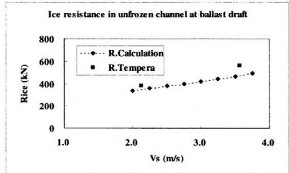
Figure 15: Comparison ice resistance of selected hull form in unfrozen channel at ballast draft in astern with existing DAT "Tempera" <sup>(4)</sup>
