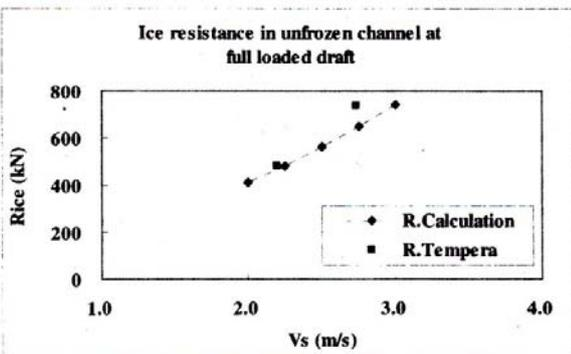
Figure 14: Comparison ice resistance of selected hull form in unfrozen channel at full loaded draft in astern with existing DAT "Tempera" <sup>(4)</sup>
