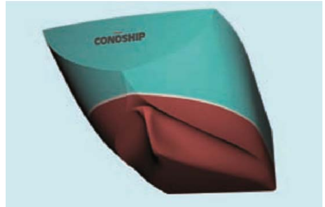
Figure 6: Moderate tunnel shaped aft ship.
