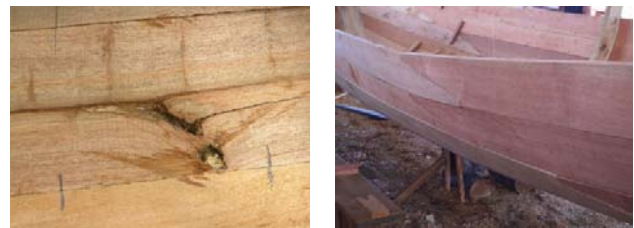
Figure.2: Quality issues in traditional ship production.
