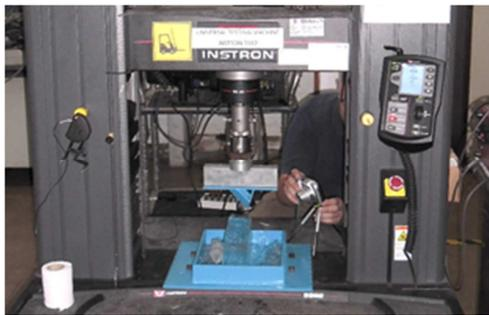
**Figure 4:** Setup equipment test on Universal Testing Machine, Instron 5982
