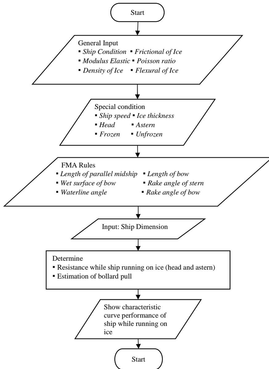
Figure 5: Main flowchart of simulation
