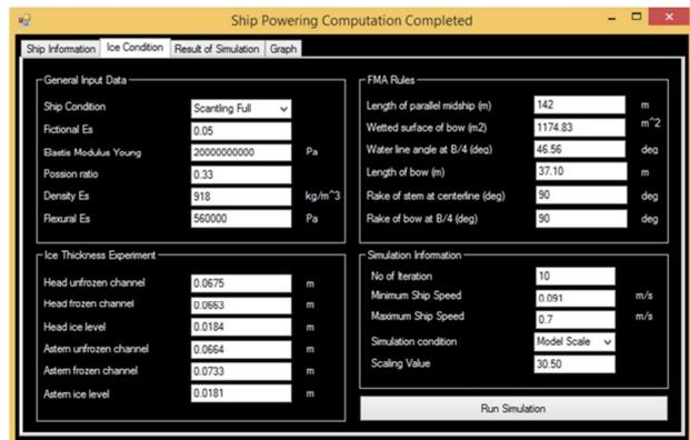
Figure 10: Ship dimension and Ice Condition to input parameters of ice.
