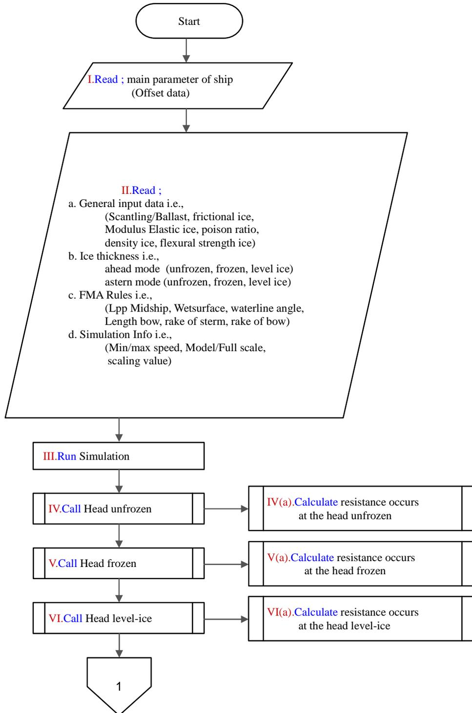
Figure 6: Simulation process for proposed method to predict resistance occurs when DAT travelling on ice at ahead mode
