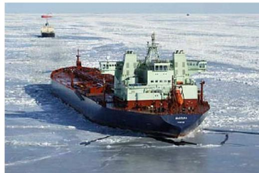
Figure 2: Double Acting Tanker in ice condition (Juurmaa et al, 2002)
