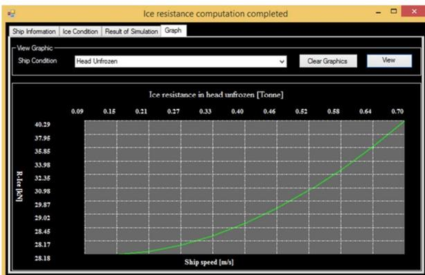
Figure 12: Result simulation in Graph, ice resistance working related to ship speed
