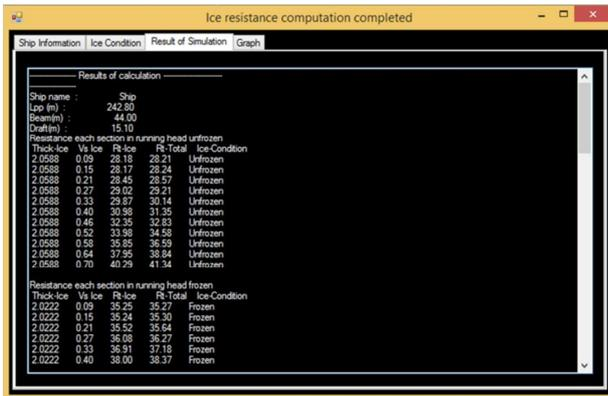
Figure 11: Tab Result of Simulation, shows classified result of simulation program
