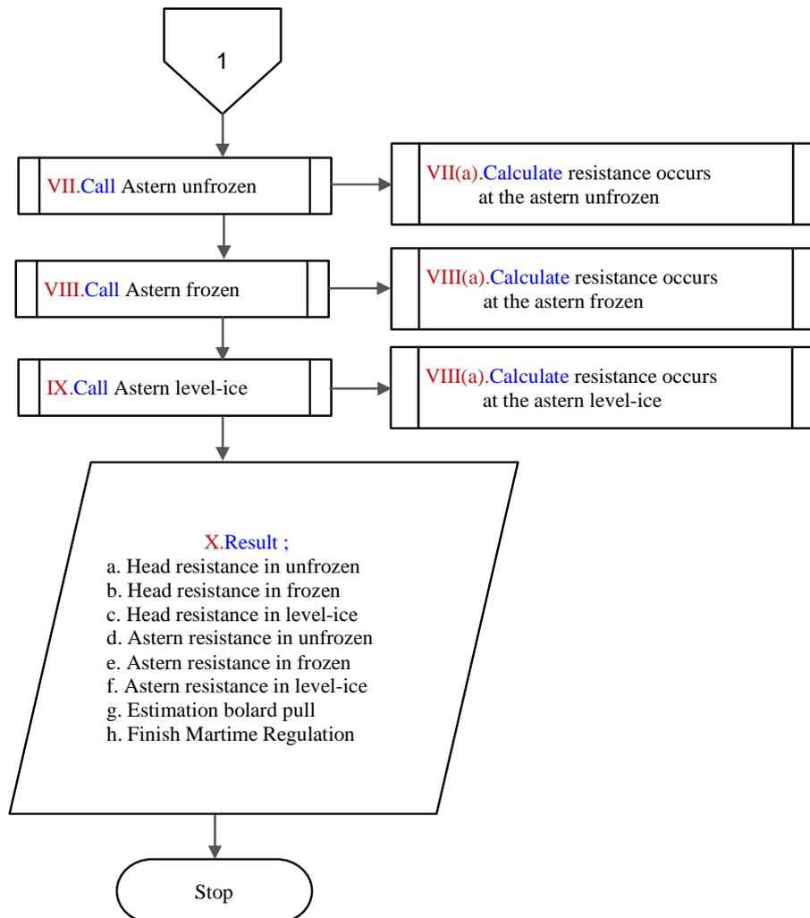
Figure 7: Simulation process for proposed method to predict resistance occurs when DAT travelling on ice at astern mode
