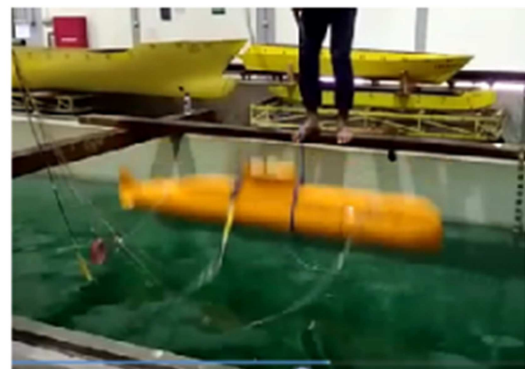
Figure 10: The submarine model was released from cable using a "release mechanism".
