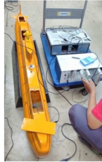
Figure 8: Accelerometer placement on Submarine Model
