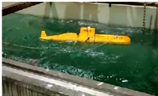
Figure 12: Submarine hydro- elastic model was on her surface draft
