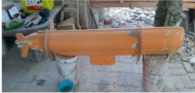
Figure 7: Installation of back-bone steel bar on the keel as submarine pressure hull elastic model
