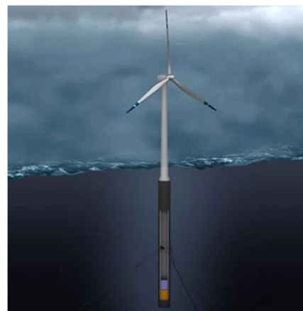
Figure 1: Offshore wind turbine floating with Spar buoys
