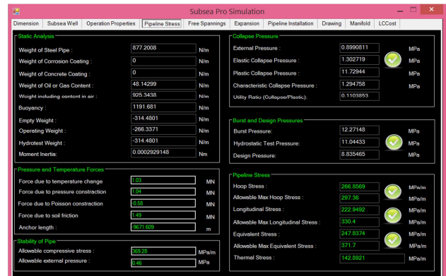
Figure.2: Wall thickness and stress analysis using Subsea Pro Simulation.
