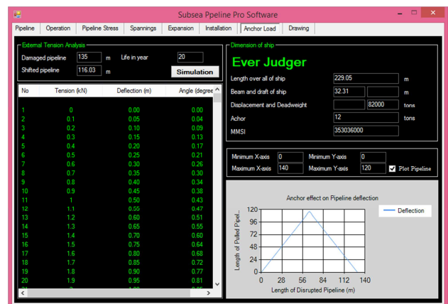
Figure 10: Anchor effect on subsea Pipeline
