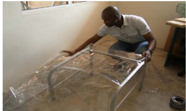
Figure.3: Constructing the Air Drying model.
