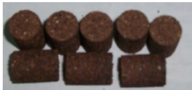
Figure 2: CNS pellets using starch as a binder.
