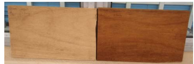
Figure 10: Effect of rainfall on drying of lumber using the proposed technique and traditional technique.
