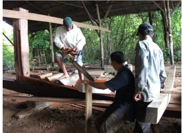
Figure 7: Unsafe condition when cutting the wood.
