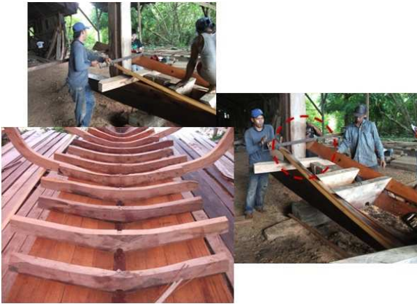
Figure 9: Planks fastening at bottom frames of ship.
