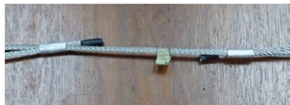
Figure 8: Example of end termination of wire rope (Siow et al., 2014)
