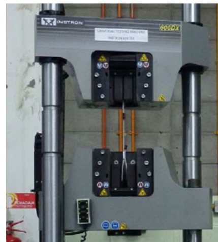
Figure 7: Tensile test machine (Siow, Koto, & Khairuddin, 2014)
