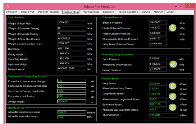
Figure.8: Subsea Pipeline analysis using Subsea Pro Simulation.
