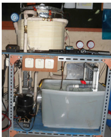
Figure 2: Apparatus of freeze vacuum drying.
