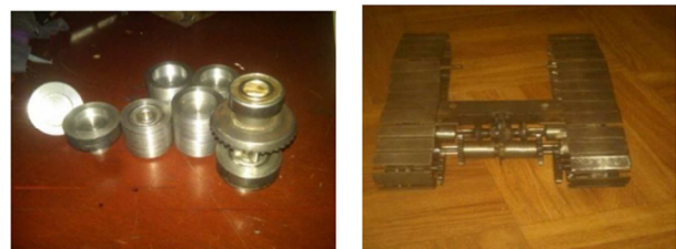
(a) The position of the gear (b) Sprocket and gear on the frame
