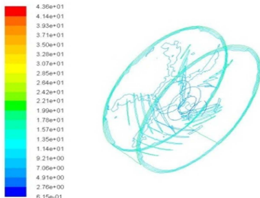
Figure 5: Contours of Velocity (m/s) of inlet, outlet, and wall solid.
