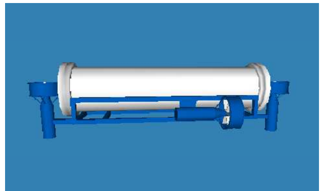
Figure 5: The one-hull, four-thruster concept design.
