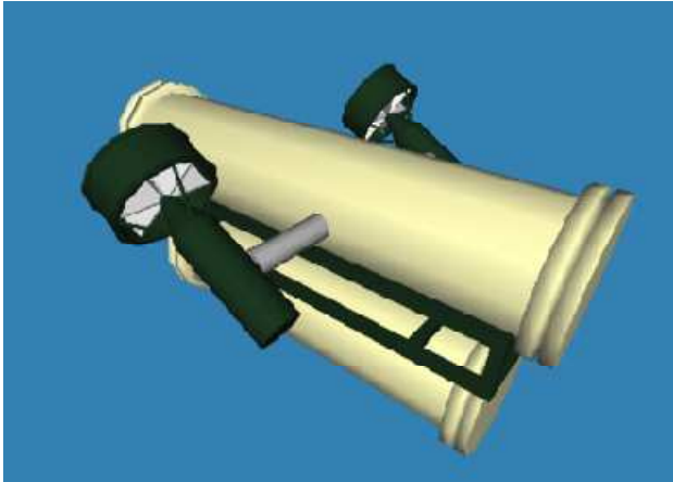
Figure 7: The two-hull, rotational thrusters concept design.
