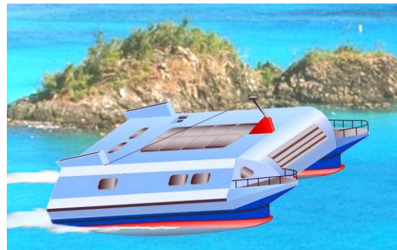
Figure 4: Semi-planing SWATH as a mini-ferry or motor yacht.
