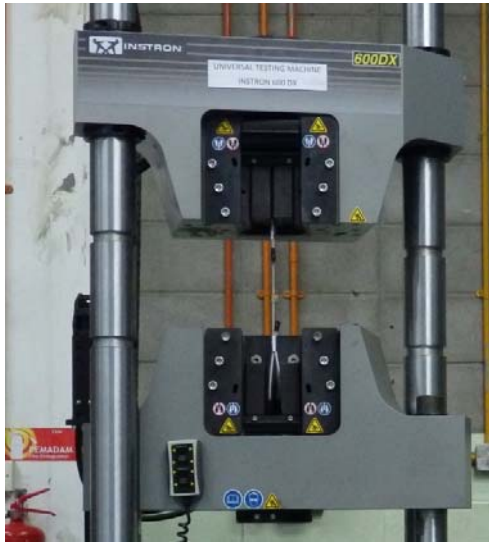
Figure 5: Wire rope tensile experiment setup
