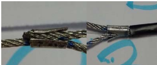
Figure 6: Sample of failure tensile experiment due to breaking of end termination.
