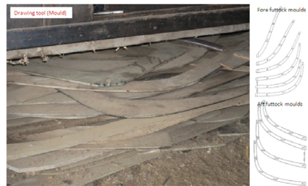
Figure.6: Molds used as guidance for frame shaping.
