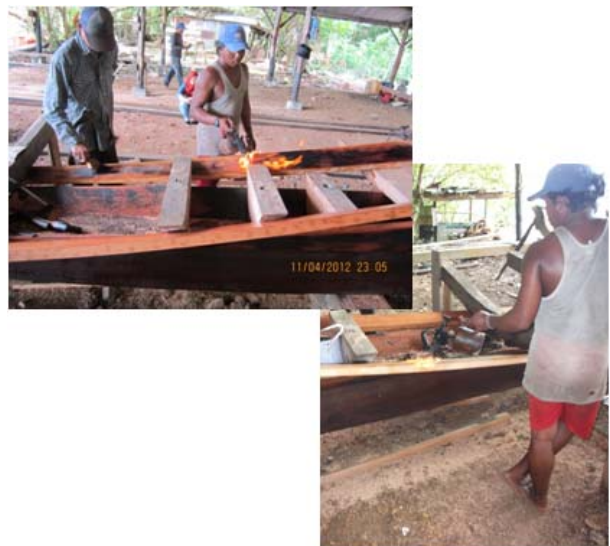
Figure.16: Planks bended using fire technique
