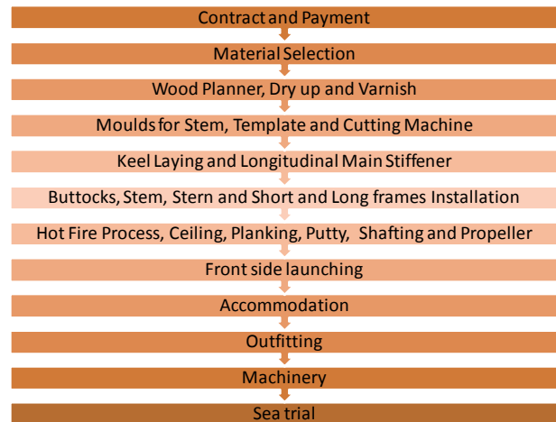
Figure.3: Flowchart of traditional shipbuilding process.
