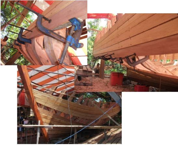
Figure.14: Upper planks assembled to vertical frame
