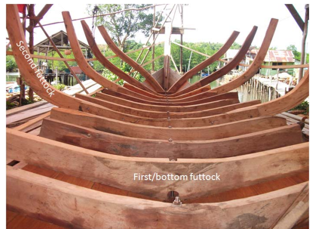
Figure.9: Typical example futtocks installed in traditional ship.
