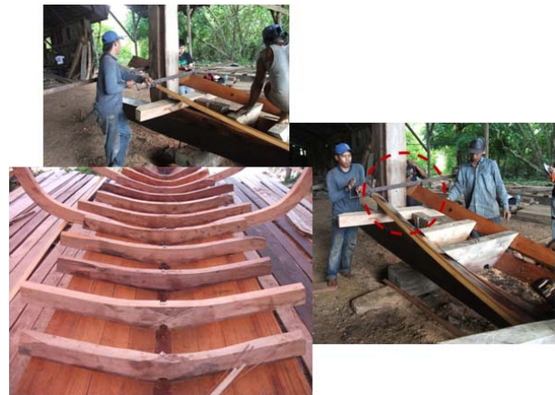
Figure.15 Planks fastening at bottom frames of ship.
