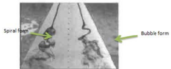
Figure 2.2: Form of vortex breakdown (courtesy from Study on Forms of Vortex Breakdown over Delta Wing. Chinese Journal of Aeronautics, Vol. 17 No 1, 2004).
