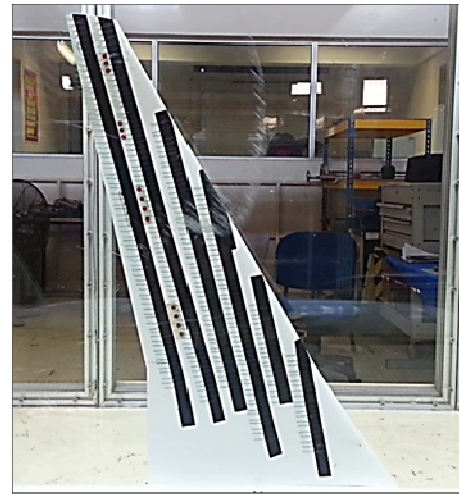
Figure 4: Threaded tuft used as a flow visualization method
