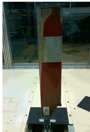
Figure 6: Gap between tail rotor blades with wind tunnel floor.
