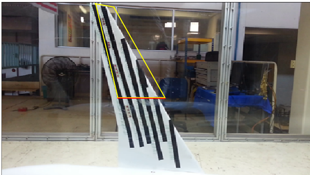
Figure 12: Flow visualization using threaded tufts at \alpha = 10^\circ at Re = 1.5 \times 10^6
