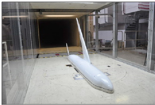
Figure 3: The installation of UTM half model attached to a semi span balance in UTM LST
