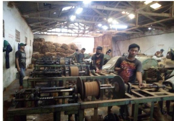
Figure 5: A simple spinning m/c for coir rope
