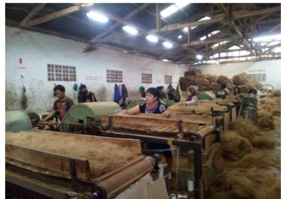
Figure 6: Coco fibers feed into spinning m/c
