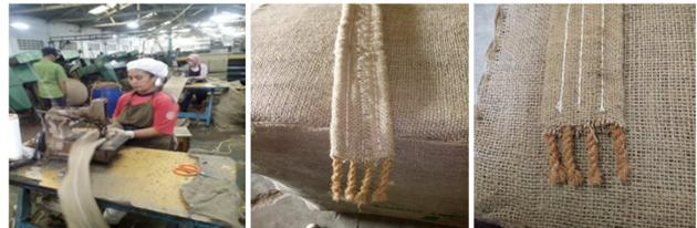
Figure 7: PVD made of natural fibers, named Fibredrain.
