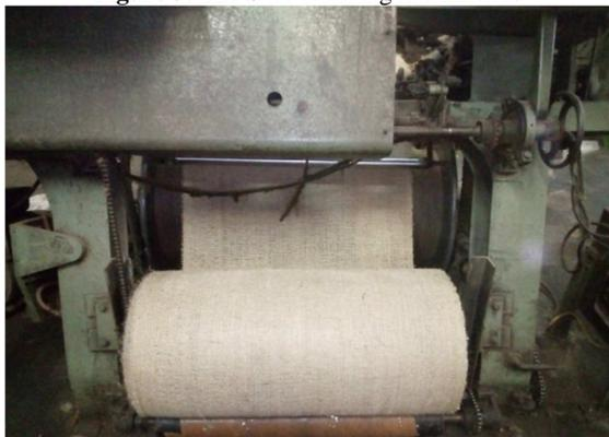
Figure 4: Jute fabric from S4A weaving m/c
