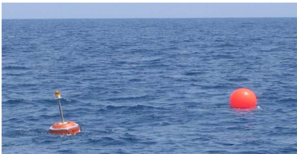
Figure 5: Wave buoy installed to measure weight height in the Merang Shore, Terengganu, Malaysia.
